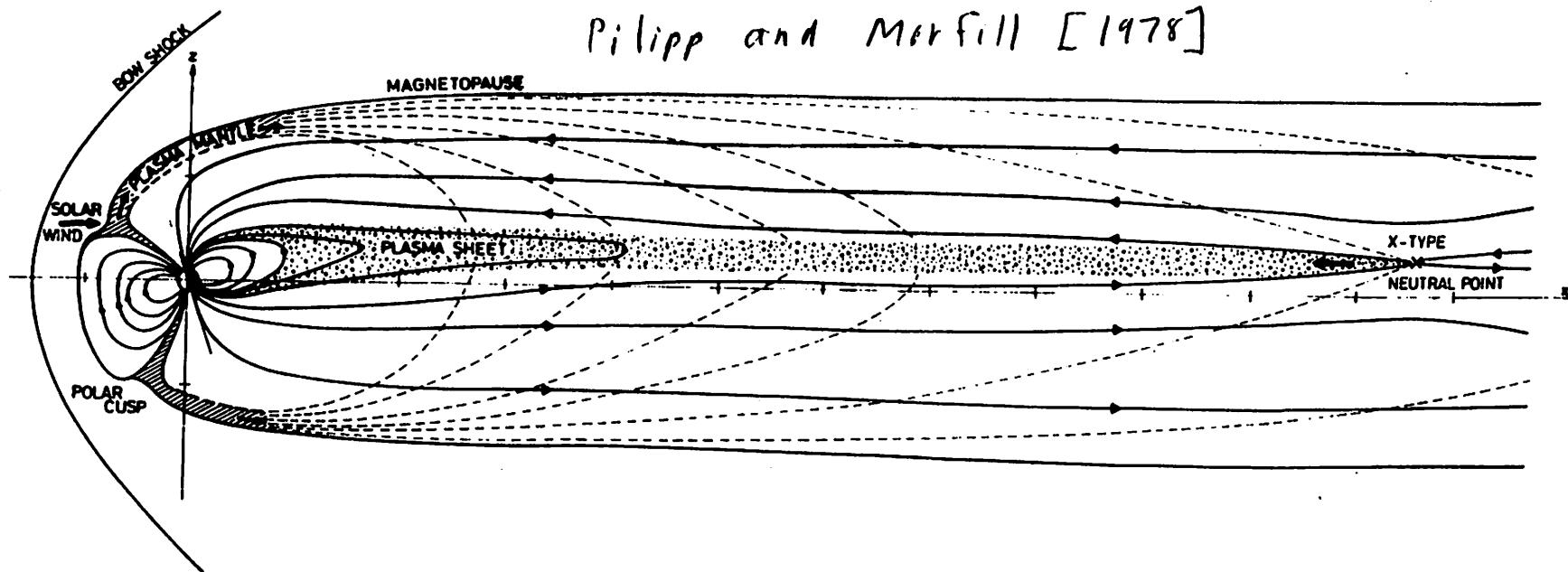
Fig. 1. Schematic diagram of the transport of mantle plasma onto the plasma sheet under the influence of the large-scale convection electric field. The mantle particles disperse and move along the dashed lines. Mantle plasma entering the field reversal region within the 'neutral point' becomes trapped and forms the plasma sheet. The magnetic field (solid lines) is depicted as an instantaneous snapshot of the quiet time configuration.
