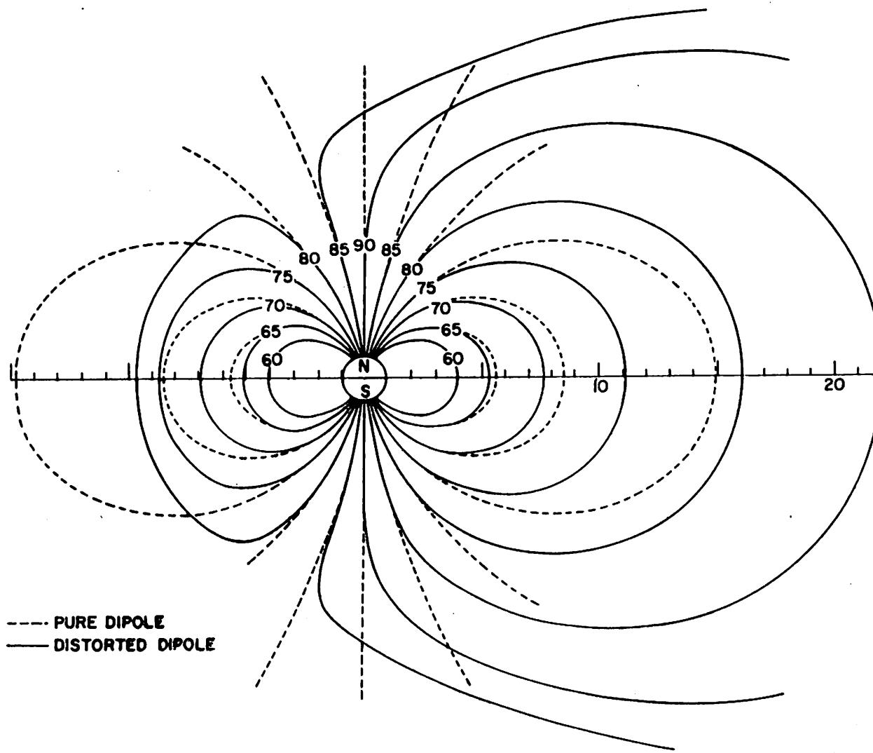
Fig. 4. Field line configuration in the noon-midnight meridian plane. With  $r_s = 10$  earth radii, the critical latitude is about  $83^\circ$ . The dipole lines are compressed on both the daytime and nighttime side.
