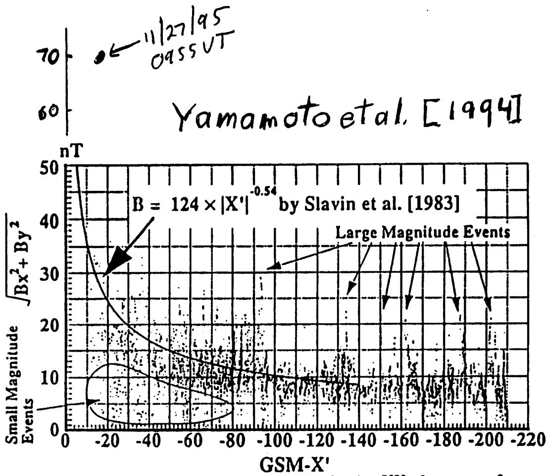
Figure 3. Magnitude of magnetic field in the XY plane as a function of  $X'$ . The empirical curve by Slavin et al. [1983] is drawn as a reference.
