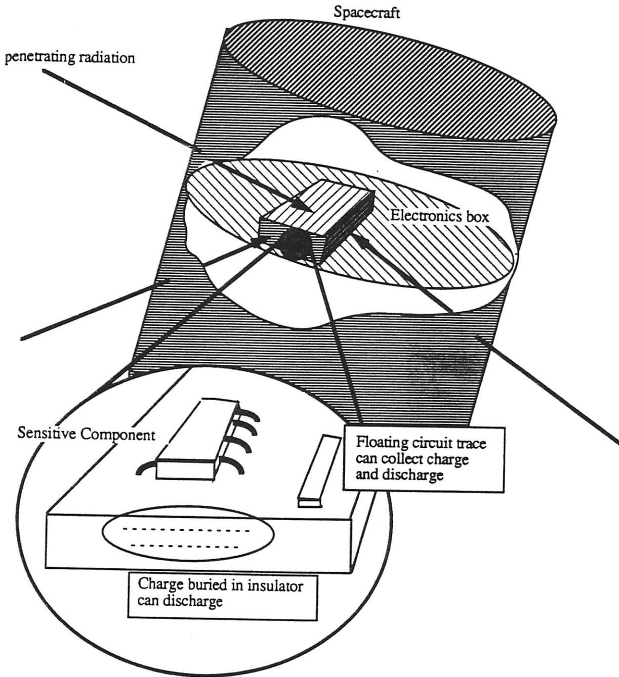
Figure 1-4. Internal Discharges Result From Charges Deposited Directly On or In Well Insulated Regions Inside the Spacecraft
