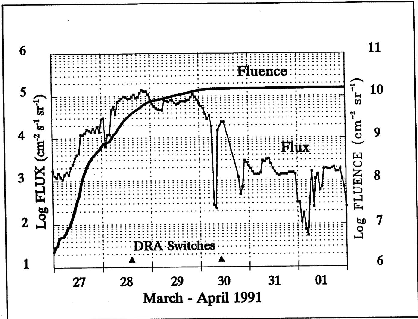
Fig. 6 Flux and fluence of  $> 2$  MeV electrons measured at GOES-7 during 6 days in March-April 1991; times of the first two  $DRA\delta$  ATC/IFC switches are shown.
