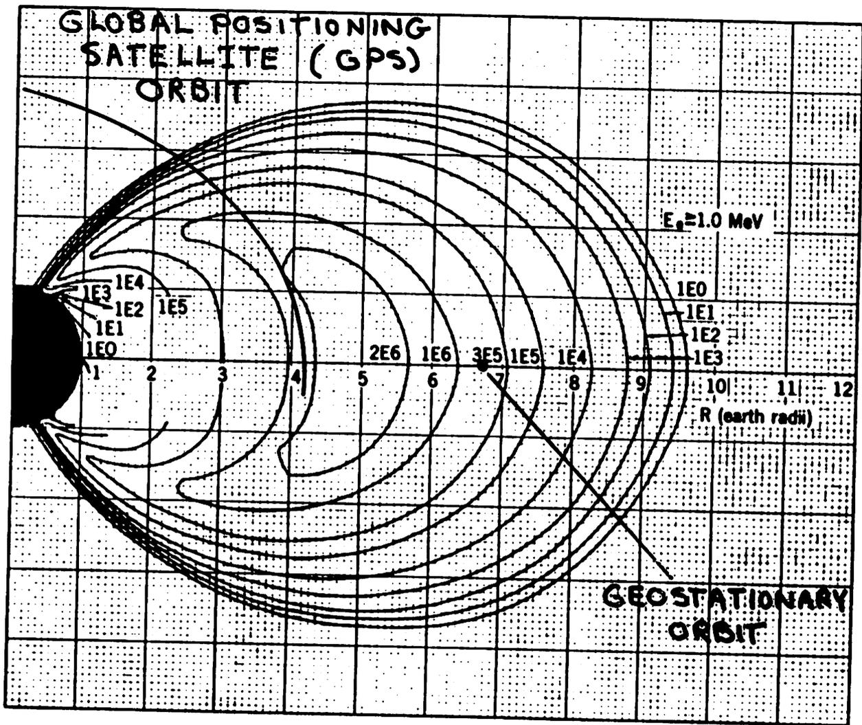
R-λ Map of AE-4 Electron Fluxes for Epoch 1964, Threshold Energy 1.0 MeV
