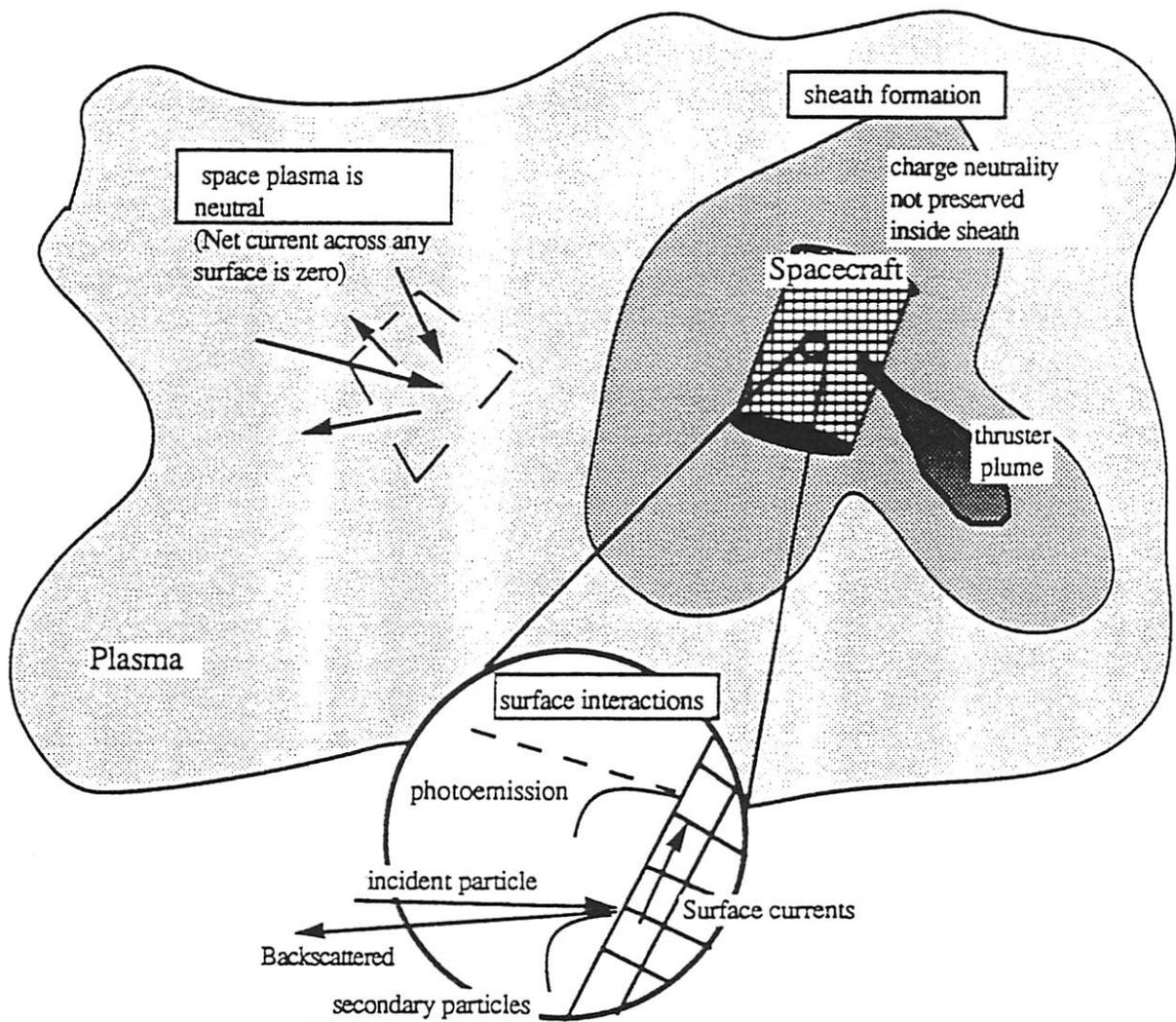
Figure 1-2. Surface Discharges Result From Charge Built Up on the Surface of the Spacecraft.
