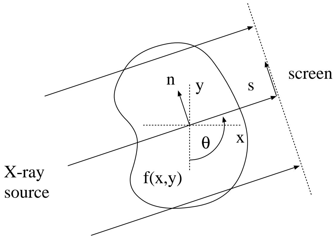
$$\begin{aligned} d(\theta, s) &= \int \int m(x, y) \delta(x \cos \theta + y \sin \theta - s) dx dy \\ \hat{d}(\theta, k) &= \hat{\hat{m}}(k \hat{n}_\theta) \end{aligned}$$
