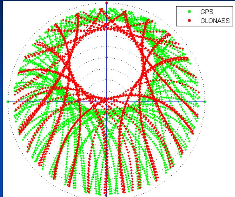
GLONASS orbit plane inclination:  $65^\circ$
