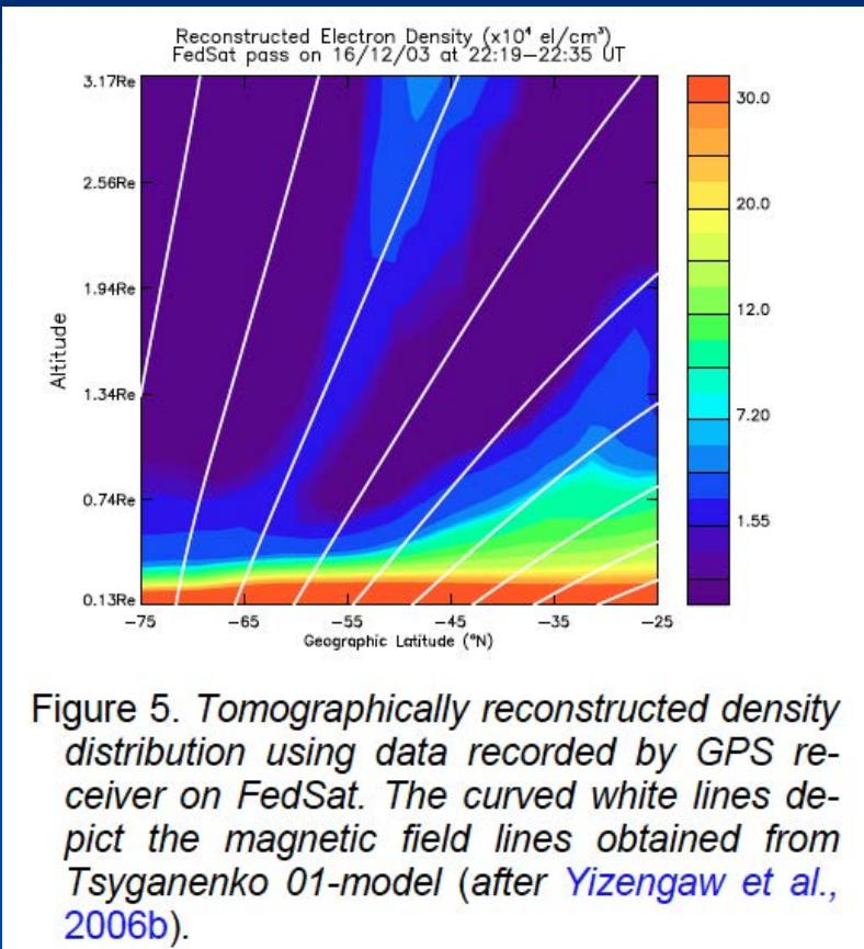
Figure 5. Tomographically reconstructed density distribution using data recorded by GPS receiver on FedSat. The curved white lines depict the magnetic field lines obtained from Tsyganenko 01-model (after Yizengaw et al., 2006b).
