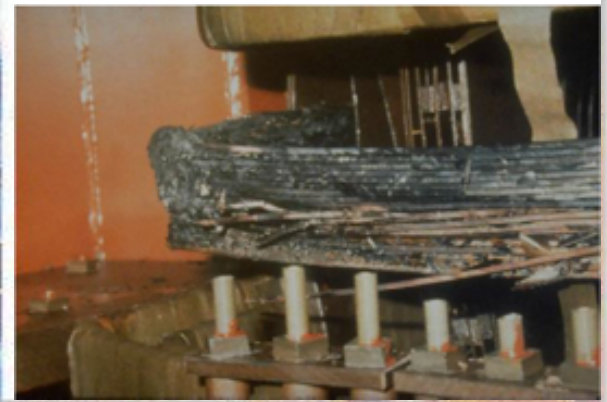
A large space storm in 1989 caused currents which damaged this transformer and shut off power for six million people for nine hours.
