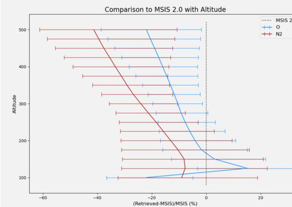
Early comparisons to MSIS 2.0 suggest that retrieved O and N<sub>2</sub> densities are systematically low (this is consistent with high O/N<sub>2</sub>). The increased discrepancy with altitude indicates that we have a smaller retrieved scale height.
