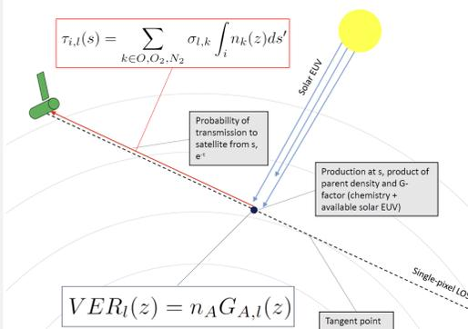
We model the EUV emissions under production by solar and photoelectron excitation and transport with pure absorption by neutral O, O<sub>2</sub>, and N<sub>2</sub>. We scale condition-dependent G-factors for 83.4 nm and 108.5 nm to model production. We use cross-sections from Conway (NRL) to calculate absorption.
