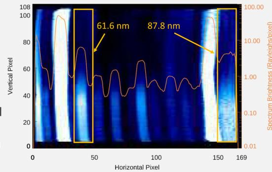
The instrument measures the F-region ionosphere using O<sup>+</sup> airglow at 83.4 nm and 61.6 nm. Both are produced by solar photoionization of O, but the former scatters off O<sup>+</sup> while the latter is optically thin. In addition to these two features, the EUV instrument measures airglow profiles at 10 other wavelengths, including a band near 87.8 nm. (Sirk et al. 2017).
